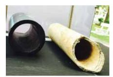
HDPE (left) and Asbestos Cement
